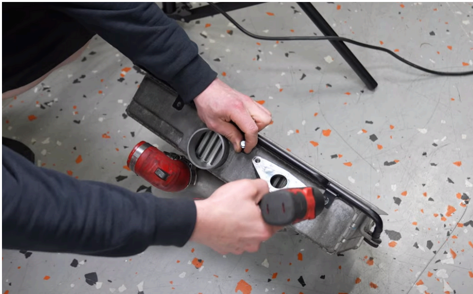
Step 11 Remove the crossover pipe from the intercooler.
